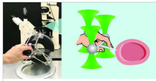
Conceptual representation of a highly nimble micromanipulation experimental setup. Cells can be explored with advanced laser trapped microtools that extend the operator's sense of touch thanks to a specifically designed haptic teleoperated optical tweezers.
